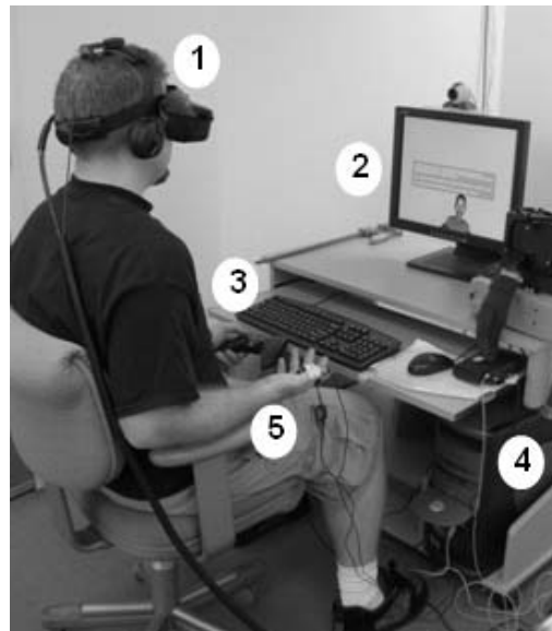
Figure 2: Participant in VR learning environment: 1) Head-Mounted Display (HMD) and orientation tracker, 2) monitor showing the experimenter what participant is seeing in the HMD, 3) Game-pad used to notify agent/avatar, 4) rendering computer, 5) equipment recording skin conductance level (SCL).
